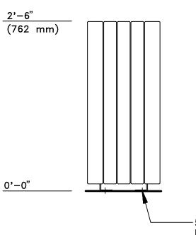
5/8" (16 mm) DIAMETER HOLES PROVIDED FOR ANCHORS BY OTHERS. (TYPICAL-4)
